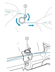
Thread guide for bobbin winding 1
